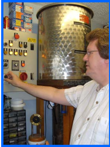
An Hot Liquor Tank being fired up!
